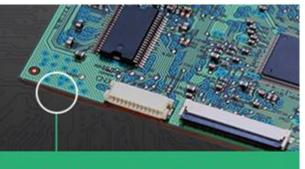
Boards with **greater thickness** will offer more support when heavy connecting objects need to be supported.
