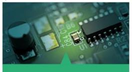
The silkscreen layer makes it easier for electronics assemblers to place each PCB in the proper place and in the right direction on each component.
