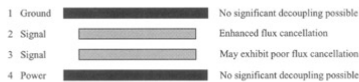
Figure 2.12: Four-layer stackup assignment—alternation configuration.
