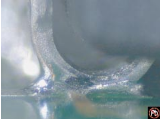
Figure E-7 SnAgCu Solder; No Clean Process, N2 Reflow
